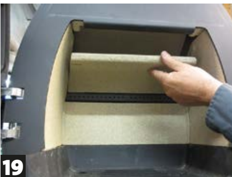
16 Push the plate upwards so that it rests on the front plate
